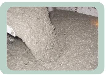
Wet shotcrete admixtures include a set stabilizer, flow enhancement admixtures, and high-performance accelerators.
