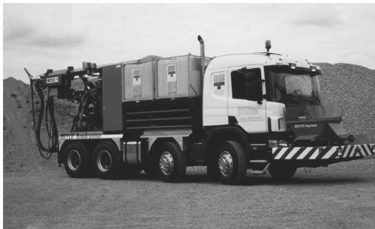
Figure 49: MEYCO® Roadrunner 2000: This mobile spraying system contains all specified equipment of the MEYCO® Spraymobile, mounted on a roadworthy truck. All equipment can be powered either from an external source or by its own Diesel motor. In addition to the MEYCO® Spraymobile it also contains a tank for curing agent.
