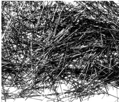
Figure 23: Steel fibres as used for reinforcing of sprayed concrete for rock support
