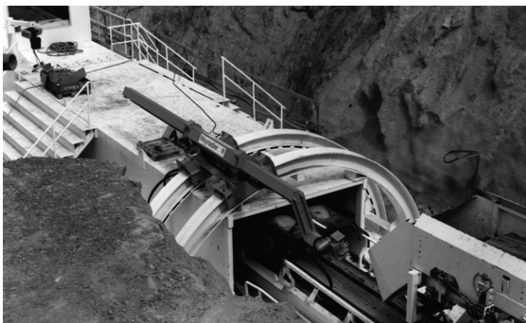
Figure 43: Tailor-made solution by MBT: The MEYCO® Robojet spraying manipulator is integrated into a large diameter TBM.
