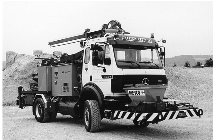
Figure 12: The sprayed concrete in the Heliopolis tunnel, which is part of the Belo Horizonte Metro, was applied through a MEYCO® Roadrunner.
