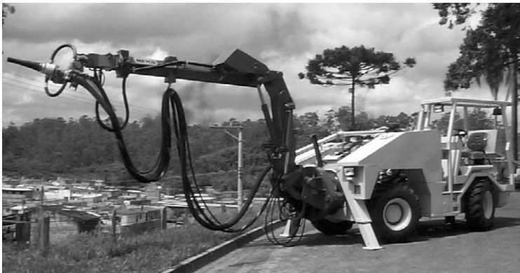
Figure 48: MEYCO® Mamba Spraymobile: Mining version.
