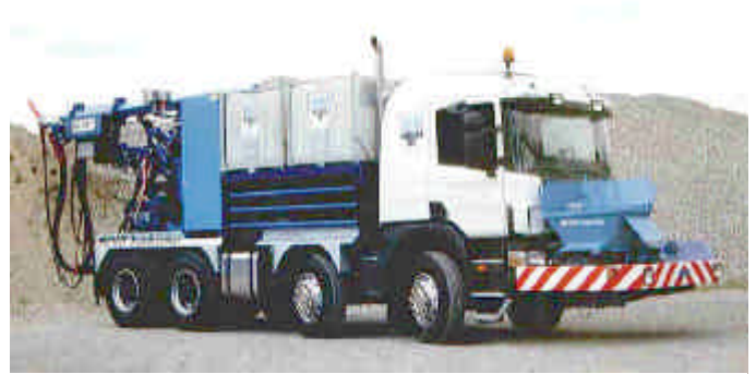
Figure 18: Meyco Roadrunner - road worthy spraymobile
