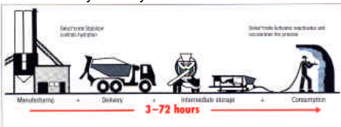
Figure 8: Hydration control for total flexibility in sprayed concrete
