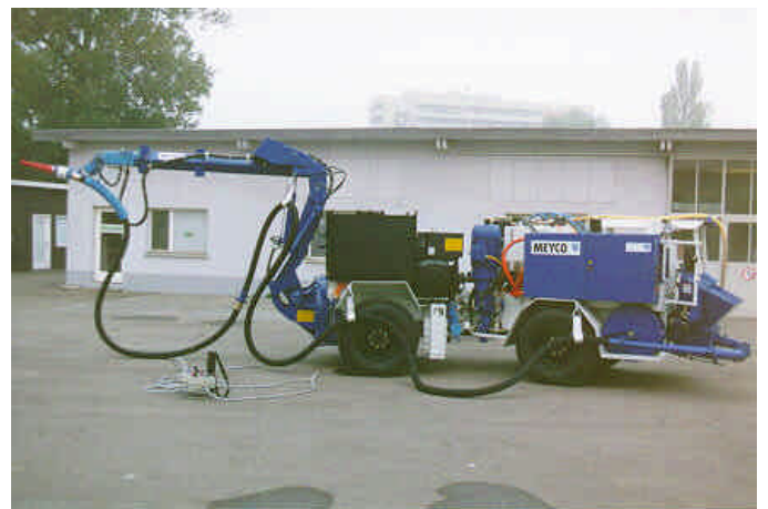
Figure 19: Meyco Cobra - Mining industry spraymobile
