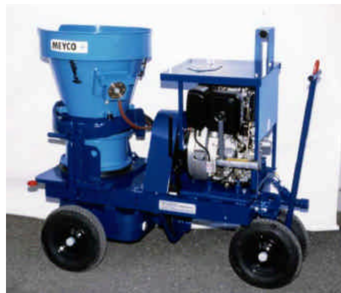
Figure 2: Typical dry-mix sprayed concrete pump
