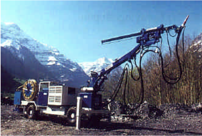
Figure 17: Meyco Spraymobile – complete sprayed concrete system on board vehicle
