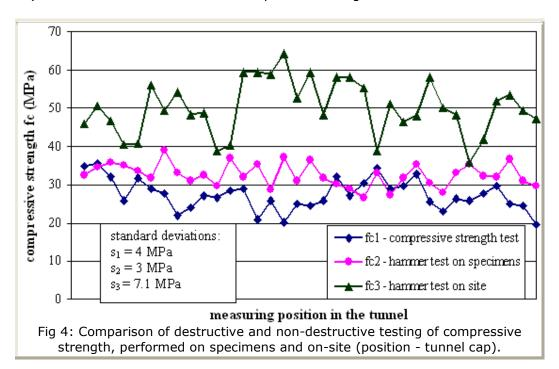
In conclusion, only the use of the non-destructive and destructive test methods for determining the quality of concrete makes it possible to estimate the quality of the built structure in a practical manner and with sufficient accuracy.
