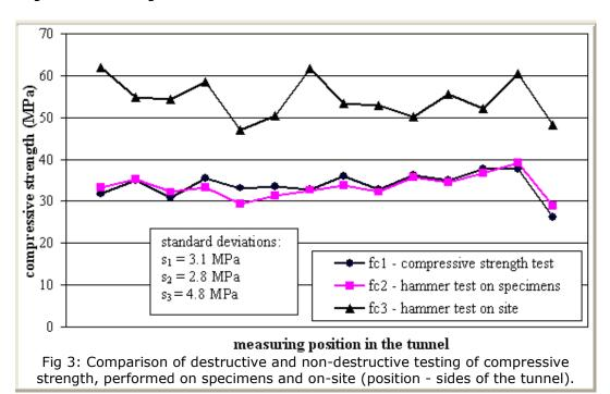
Figure 3 and Figure 4 shows that the use of the hammer test method along the tunnel primary lining gave significantly higher values and higher standard deviations than the use of the same method along the drilling cores taken out of the structure. The analysis
